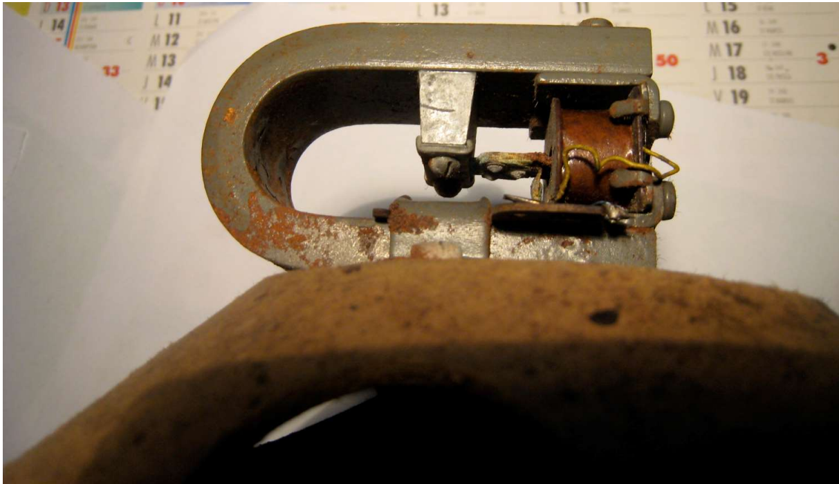
Figure 11- Electroaimant du HP
